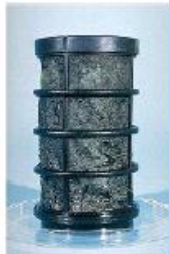
Plugged fuel filters
