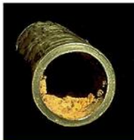
Build-up of sludge in fuel lines and restricting flow
